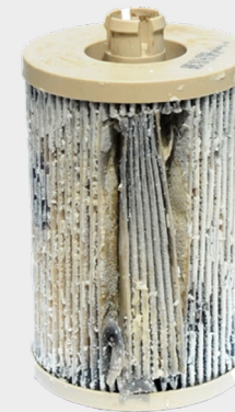
Figure 33 Use of biodiesel of inadequate quality in fuel blends can have negative operational implications
