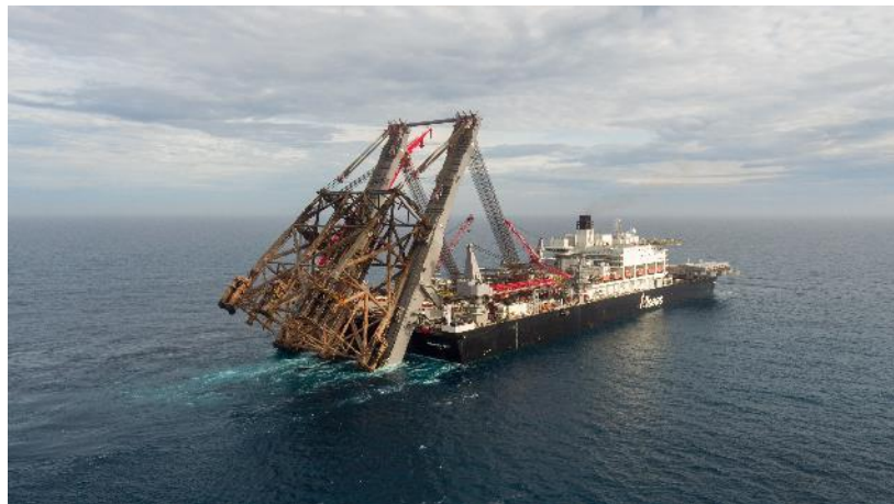
The Heavy Lift Vessel Pioneering Spirit with a removed jacket onboard
