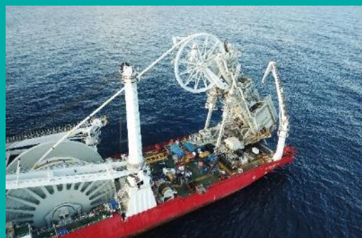
Example of the reverse reel-lay removal method (Source: Subsea7)
