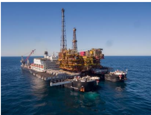
The Allseas Heavy Lift Vessel Pioneering Spirit lifting the topsides of a platform on a previous project
