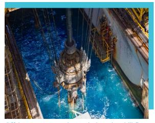
Offshore moon pool area below the drill floor. Within the moon pool, centrally shown is the marine riser with slip joint and tensioner lines.
