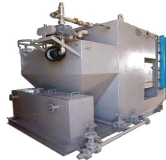
**Food Waste Treatment**—For vessels located >12 nautical miles from shore, food wastes can be treated through a shredder or a macerator and pass through a 25-millimeter mesh screen prior to overboard discharge. Food waste discharge must be visually monitored to ensure there are no floating solids after treatment. Food waste treatment is conducted in batch mode when required.
