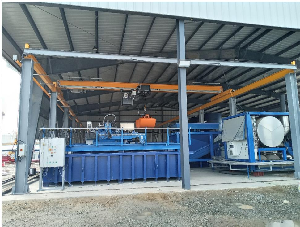
**Figure 6-15: Incinerator unit**
